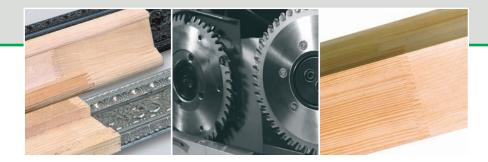
This line ensures a uniform, precise cutting pattern all over the entire package width by frequency-controlled cutting table motors with high infeed power.
