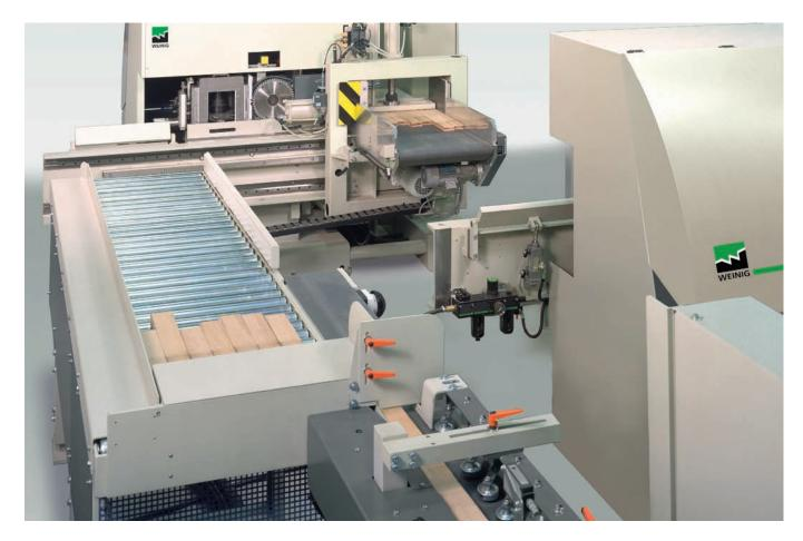
By the modular design of a finger jointing line you have the possibility to determine the degree of automation yourself. No matter whether you wish to operate a manual, a semi-automatic (including separating magazine) or a fully automatic line: Depending on the requirements WEINIG GRECON recommends the right degree of automation.
