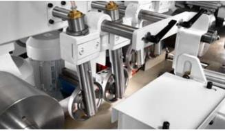
Double top pressure rollers opposite the left vertical spindle, are moved together with the tool.
