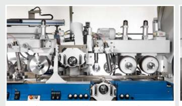
The short feed roller distance (less than 1.200 mm) and the large feed roller diameter (250 mm), results in good transportation of short pieces.
